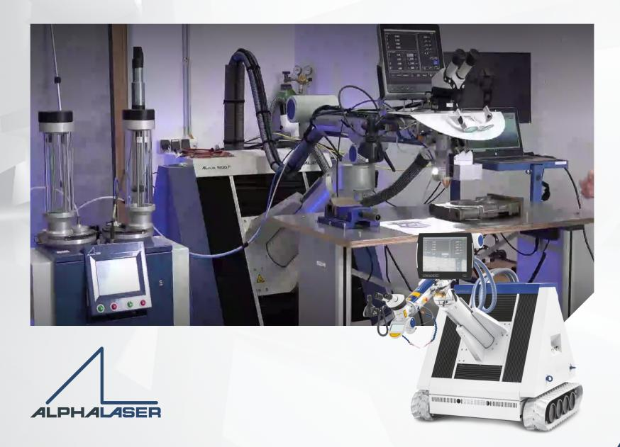
New Alpha Laser AL Flak 1200 Fiber Laser with Mabotix Scan Camera to create 3D Files for Additive Manufacturing repair processes.
