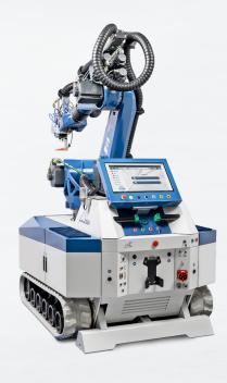
The laser beam precisely follows the workpiece contour in free 3D movements. This makes it easy to harden closing edges, grain structures, dimples or individual points.
