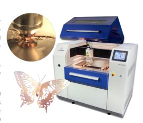
The fully automatic cutting process takes place in the closed, laser-safe working chamber and can be observed through a large protection window. The system is operated via the intuitive touch screen.
